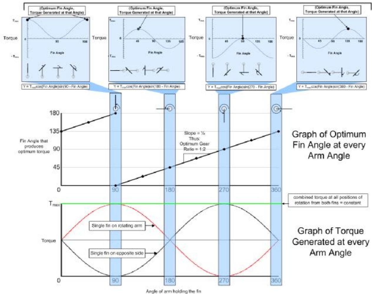
A common question that is asked of this design is, “Why don’t you curve the fins?” There are two reasons that the fins are flat. One reason is that at the lowest position when the sail is moving against the flow of water, a curved sail would have drag. Another reason is that because the fins turn at half the speed of the main rotation so
