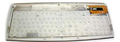
This keyboard uses rubber dome switches.
