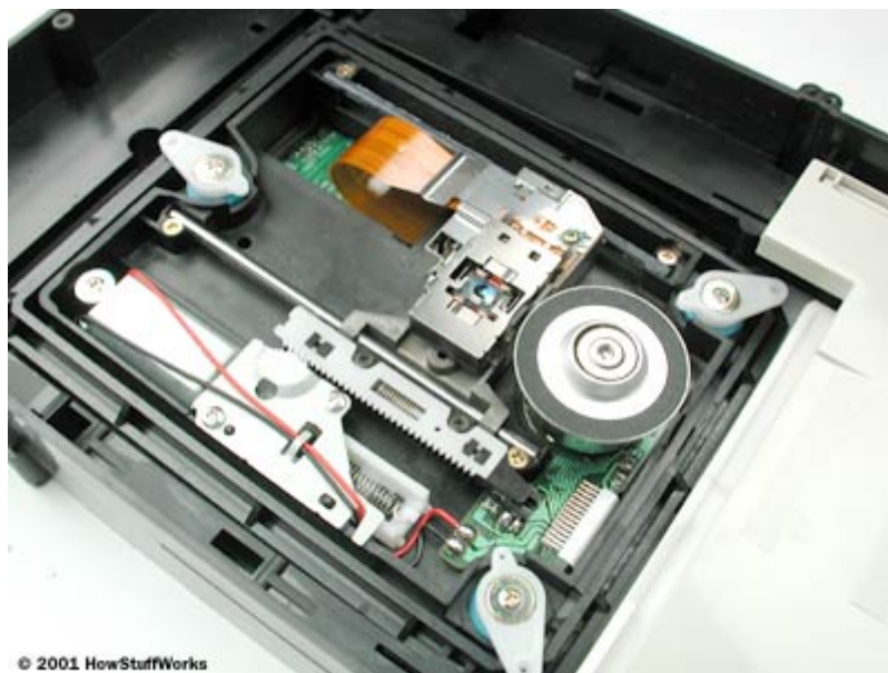
The machinery in a CD burner looks pretty much the same as the machinery in any CD player. There is a mechanism that spins the disc and another mechanism that slides the laser assembly.
