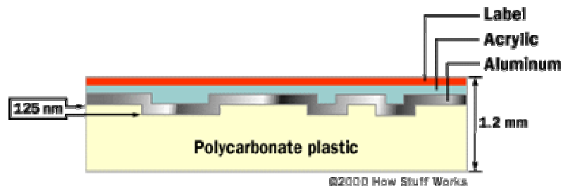
The different layers of a conventional CD
